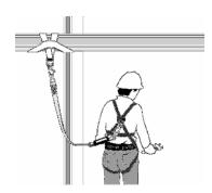
The anchorage point can be a single attachment to a substantial structure above the surface from which the employee is working, or it can be one to two attachments used to anchor a vertical or horizontal lifeline.
